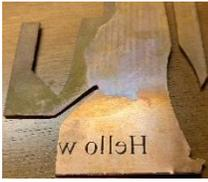
Clean off all oxide with an abrasive pad or with very fine steel wool and wipe down with acetone. Let it fully dry before proceeding.
