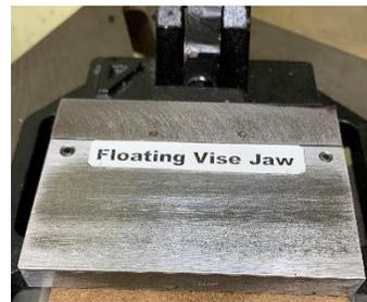
Using toner transfer, those labels can look as professional as what comes out of your laser printer plus will be far more durable. Here we have toner transferred onto powder coated aluminum which has been glued onto the surface of the tool.
