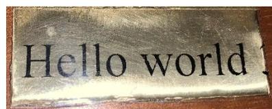
By printing on the back of clear plastic, I was able to flip it over and glue the coupon down. The result is toner sandwiched between the base metal and a covering of plastic. Now that is rugged.
