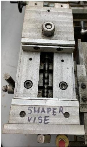
No matter how nicely you make something in your shop, it will look less than professional if the label attached to it looks ratty. Consider a superbly machine shaper vise labeled with a permanent marker. Ouch! Equally bad is a slip of paper glued in place, especially when it gets smeared with grease.
