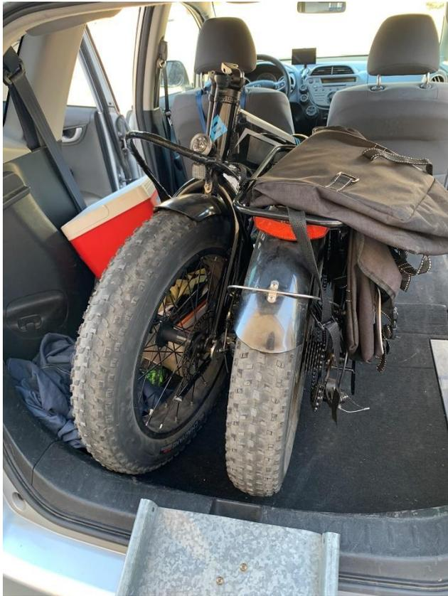
To unload the bike, I roll the back wheel over the lip of the hatch and onto the ramp. Then I pivot the bike, so the third wheel clears the lip and then rolls down the ramp.
