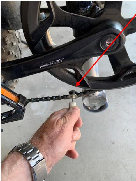
Before folding the bike, I place the tool on the chain just before it enters the front sprocket. As I turn the crank, I push. This guides the chain off of the gear.
