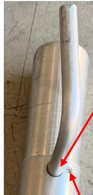
Then I cross-drilled a 3/8 inch hole just below the transition to full diameter.
