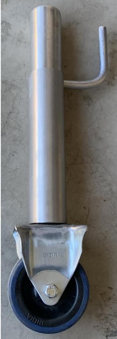
The removable third wheel consists of a fixed wheel secured to the bottom of a thick aluminum rod. An arm extends out the back, which engages with a hole in the bike's frame to prevent the assembly from pivoting.
