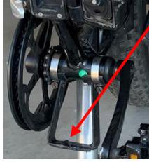
When folded, the bike rests on the wheels and a short bail<sup>2</sup> welded to the bottom of the crank box. This arrangement works if the plan is to deadlift. It is unworkable if you are trying to roll the folded bike, particularly inside my little Honda.
