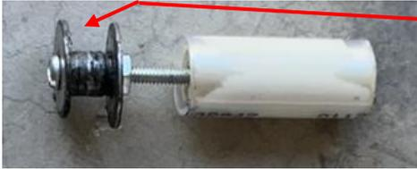
The tool consists of a pair of washers with a spacer between them. A small bolt with a nut secures them. The bolt screws into a threaded cylinder I found in my junk drawer. The spacer is slightly wider than the bike's chain.
