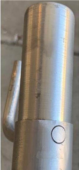
After tightening the setscrew again, I trimmed off the excess rod, so it was flush with the cylinder.
