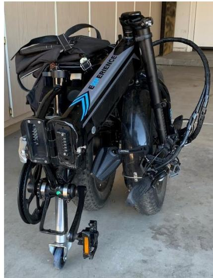
Since the crank is not connected to the chain, I can now smoothly roll the folded bike forward and backward.
