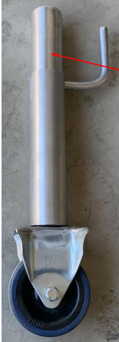
I used a length of DOM<sup>3</sup> 6061-T6 from my scrap bin for the leg. It is lighter than a solid bar stock, plus the hole lets me easily secure the wheel.
