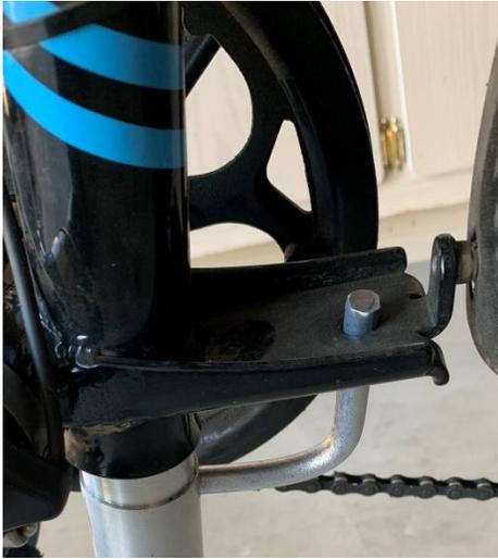
I loosened the setscrew. With the cylinder in the down tube, I adjusted the bent rod so it would enter the fender support plate with a slight flexure. This force was enough to retain the assembly until I lowered the bike onto the wheel.
