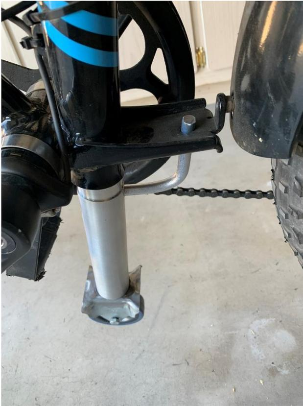
The rod has just enough spring to slide through the existing hole in the rear fender support and lock into place.
