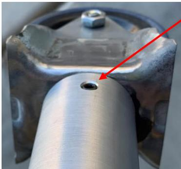
Next, I drilled and tapped a 1/4-20 hole near the bottom of the leg. The installed setscrew locked the mounting post after I had roughly aligned the wheel to the major axis of the bike.
