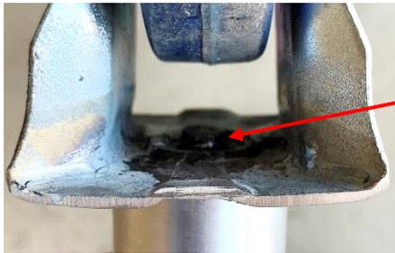
I found a bit of scrap steel that was a close fit to the axial hole in the leg. On the end of the scrap was a 3/8 inch spigot, 1/4 inch tall which became my mounting post. With the wheel frame upright and supported on a firebrick, I fluxed the mating surfaces and then pushed the pieces together. Using a MAPP torch and some silver braze, I formed the joint. The
