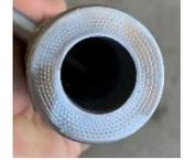
I turned down the top 3 inches of the leg for a smooth sliding fit in the bike's down tube.
