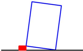
The 1-2-3 block was then tilted, so it is now parallel to the pivot shaft. Knowing the thickness of the shims plus that the block is 2-inches wide, I know the error per inch.
