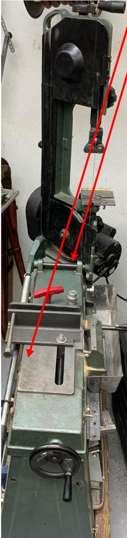
Is this machined surface on my 4 x 6 bandsaw parallel to my pivot shaft<sup>2</sup>? This is not a wildly dreamt up question. I needed to know in order to improve the cutting accuracy of my saw.
