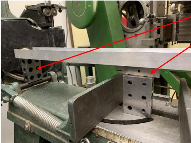
One way to figure this out is to place a 1-2-3 block between the pivot shaft and the channel. At the other end, I added an adjustable parallel on top of a 1-2-3 block.
