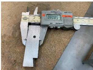
The height of the parallel *is* the distance between the outside diameter of the pivot shaft and the machined surface.
