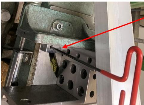
I built a sine bar and put my 1-2-3 block on top. While pushing on the channel, I adjusted the slope until there was no clicking.
