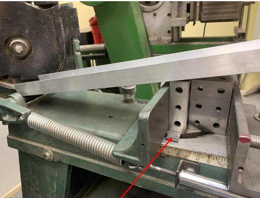
I pressed on the channel down at the pivot shaft end. This defines a line. My channel rests on the top edge of the 1-2-3 block<sup>3</sup>. Is it making contact at one point or all along this edge?
