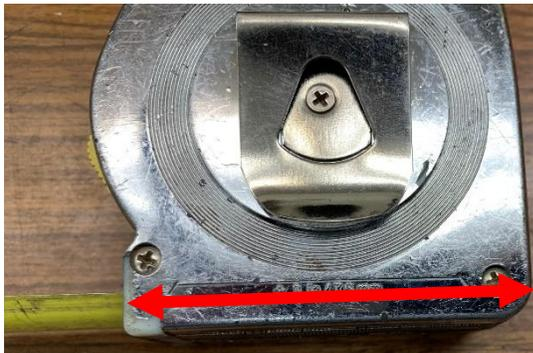
Any half-decent tape measure tells you the distance from the front to the back of the case. This old Craftsman is marked “3 in/76 mm”.
