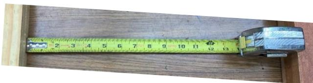
To measure inside dimensions, I feed out tape until the end touches one side while planting the backside of the tape measure against the other side.
