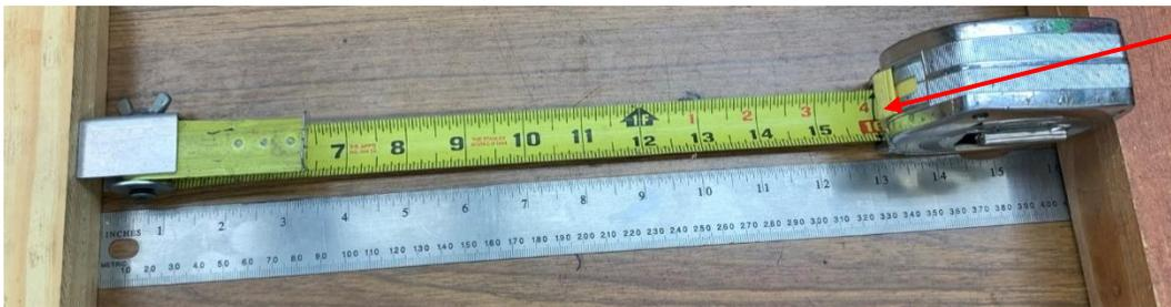
The reading on the tape measure is now the inside measurement.
