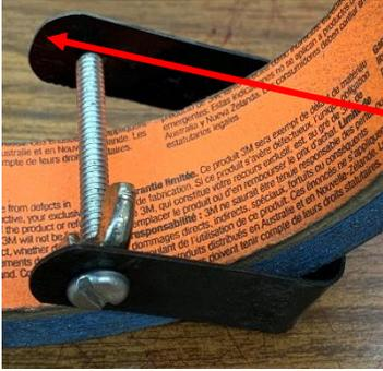
Next, use your pliers to break off the blade so the two flanks are of about equal length. Use your grinder to round the end and remove the hacksaw blade's teeth on both flanks.
