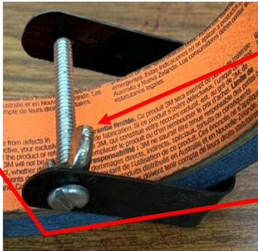
Tighten the wing nut so its ears are parallel to the inside of the roll and you are done.
