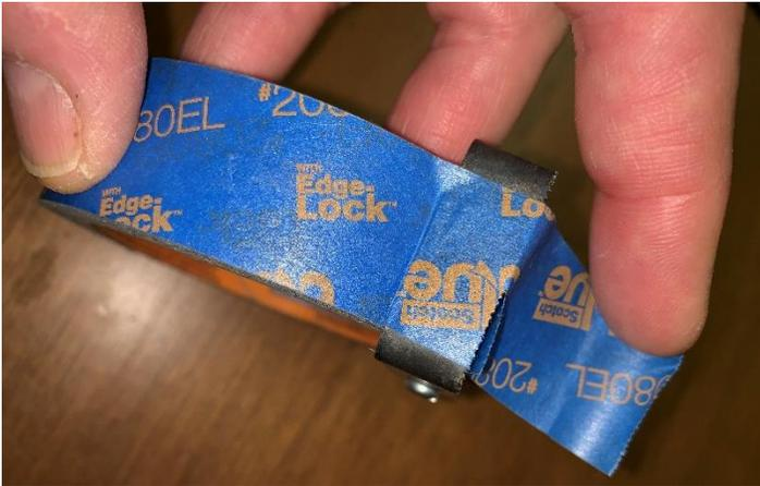
To cut, stick the tape back on the face of the blade, tilt it so the teeth point up, and pull the tape along the teeth.
