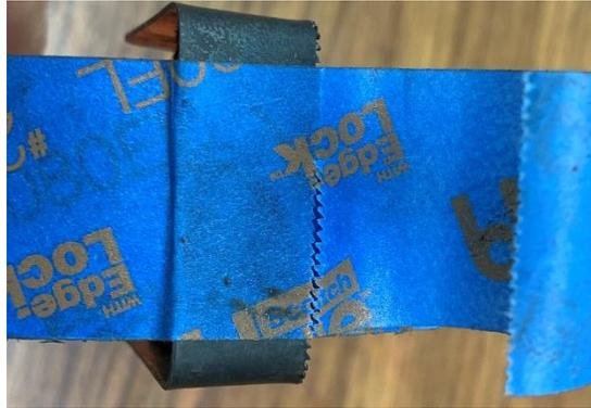
The teeth do a fine job of tearing off the tape and the face of the blade provides a surface for the end of the tape to stick.
