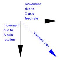
From (2) we calculated that the X axis feed rate must be 0.05 IPM.
