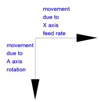
The cutter is seeing movement in two directions at the same time. As the cylinder rotates, it sees material coming at it along the Y axis. As the table moves along the X axis, the cutter sees material coming at it from this direction. There are even times when there can be movement on the XY plane causing the cutter to see a total of three different movements at the same time.
