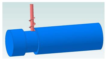
From the cutter's standpoint, it sees material coming at it as the A axis rotates. This feed rate is a function of both the revolutions per minute of the A axis and the diameter of the resulting cylinder.
