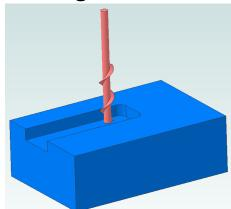
I know from experience with my RF-30 mill/drill that a <sup>1</sup>/<sub>4</sub> inch diameter 3 flute end mill<sup>2</sup> turning at 2500 RPM and cutting 0.2 inches deep in 6061 aluminum can smoothly run at 3 Inches Per Minute (IPM). Running much slower than this causes squealing as the flutes start to rub. Running much faster than this causes excessive vibration, poor finish, and in extreme cases the cutter pulls out of its holder.
