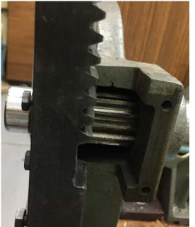
With the front cover removed from the arbor press, you can see the pinion gear and how the rack meshes with it. When the rack has been raised to where the teeth are missing, the pinion can be turned without further motion of the rack.
