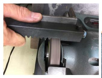
Here I am grinding off those bottom two teeth. It turns out to be the width of my bench grinder's wheel. Grind until it looks like this:
