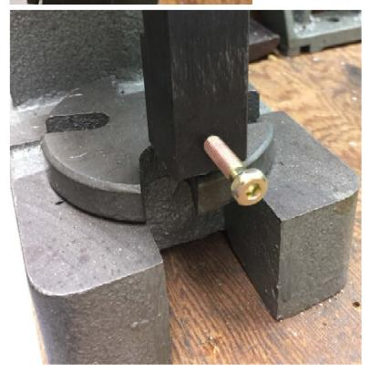
Rick Sparber <u>Rgsparber.ha@gmail.com</u> Rick.Sparber.org One minor complication did creep in. I had to replace my hex head screw at the bottom of the ram with a longer screw. The old screw head prevented the rack from rising enough to slip the pinion gear.
