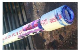
I primed the coupler and 3 inches of the pipe. Then I applied PVC cement over the same areas. In one quick move, I slid the coupler down the ½ inch pipe about 3 inches and then slid it back up to near the end. This simulated how it would be used to join two pipes. Not a lot of extra work time was available.
