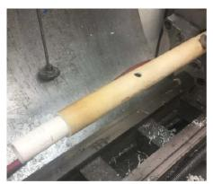
Here is a length of 1 inch schedule 40 PVC in my lathe chuck. It was heated for about 45 seconds. I forced a piece of ¾ inch schedule 40 PVC into the bore. After waiting about a minute for it to cool, the mandrel was removed. I cut off about 2 inches of the 1 inch pipe.
