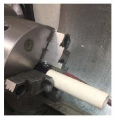
I took a 5 inch length of scrap <sup>3</sup>/<sub>4</sub> inch schedule 40 PVC and held it in my lathe chuck. The lathe was set to run at 26 RPMs. Next, with the lathe turning, I used my heat gun to warm about 2 inches of the end of this pipe. Since it was constantly turning, the heat was evenly distributed.
