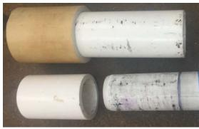
On top is the resulting 1 inch full slide coupler with a piece of  $\frac{3}{4}$  inch Schedule 40 PVC inside of it. By comparison, a  $\frac{1}{2}$  inch full slide coupler is below it along with some  $\frac{1}{2}$ " Schedule 40 PVC pipe.
