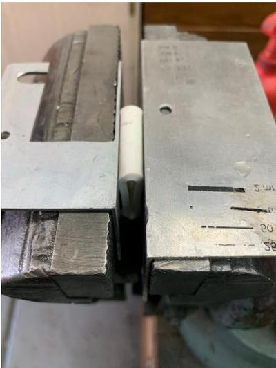
I then place the pipe into my vise and tighten it down to approximately the thickness of the straps. Once cool, the plastic will return to being hard. I speed this process along with a spray of water.
