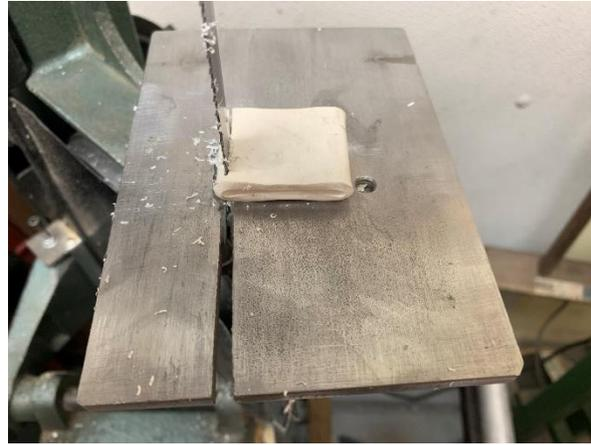
Using my bandsaw, I cut the end off of the flattened loop. The top and bottom faces of the clip are naturally aligned.
