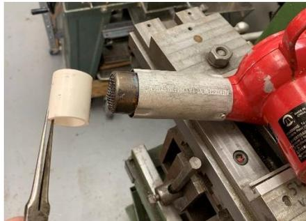
Then I heat the plastic for about 15 seconds, constantly turning it. When correctly heated, you will notice a slight slump in the pipe.
