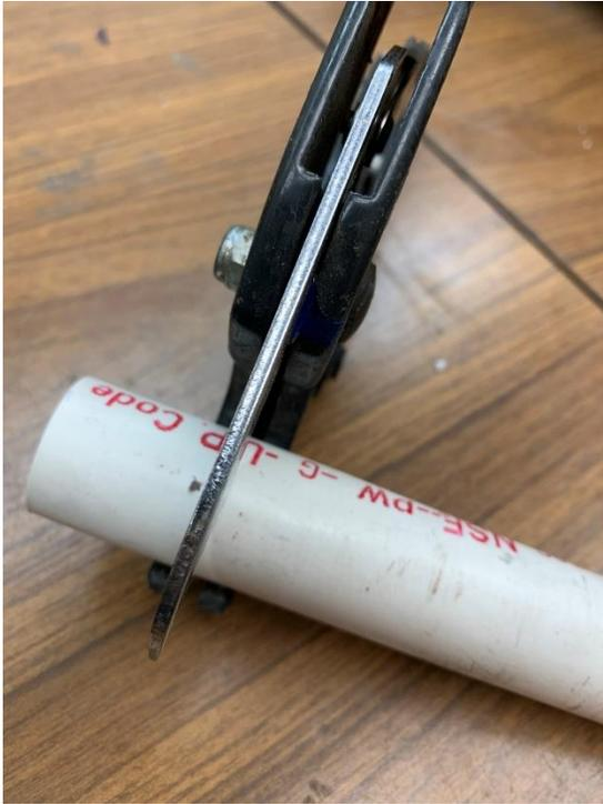
I'm using PVC snips to cut off the pipe.
