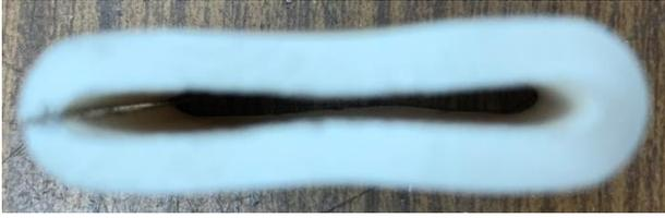
I was able to improve the clip's holding power by sawing into the end. In this example, I did not have a form inside the pipe as I reformed it. The result is a narrowing around the center. This makes installation a little more difficult but also improves the holding power.
