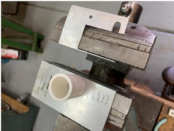
I line my vise jaws with aluminum angle and set the gap to easily pass the diameter of the pipe.
