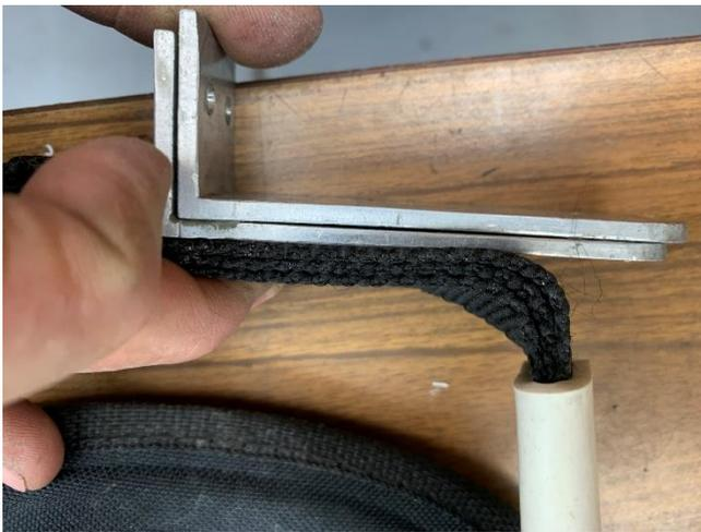
Next, I select enough scrap aluminum to approximately match the total thickness of the strap to be clamped.
