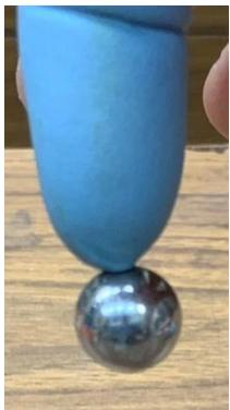
For this example, I cut a longer piece of fingertip plus changed to a neodymium magnet that was 0.1 inches in diameter and 1/16 inch thick. I was surprised that it could hold a  $\frac{1}{2}$  inch diameter ball bearing as long as I didn't move my finger too quickly.
