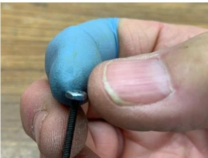
Here I am starting a #4 nut on a bolt. Picture doing this in a tight space. The magnet acts as an extra finger and prevents the nut from dropping away.
