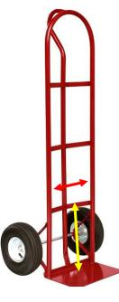
Measure the inside distance between hand truck verticals. Subtract twice the thickness of the angle and then subtract another 1/8<sup>th</sup> inch so the attachment is a loose fit.
