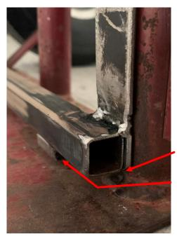
To avoid the weldment at the bottom of the vertical members, I added <sup>1</sup>/<sub>4</sub>-inch thick pads under the bottom horizontal brace.
