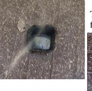
The melted square hole is rimmed with flash.
