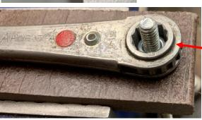
I again drill my oversized clearance hole, but this time just fit the carriage bolt. I spin on a <sup>1</sup>/<sub>4</sub>-20 nut and put my ratching box wrench over it.
