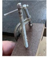
I lowered my tool through the hole and then used a MAPP torch to heat the square section until it started to glow. Yes, I'm outside, and there is a breeze, so any poisonous fumes won't get me.
