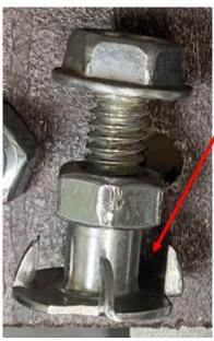
I threw together this simple tool to prevent the bolt from turning as I tightened the nut.
