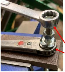
With another box wrench on the tool, I can turn the nut without the bolt turning. This enables the square section of the carriage bolt to be forced into the composite.
