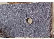
Next, I drilled a 5/32" hole. Clearance for 1/4-20 bolts is an F drill with a diameter of 0.257 inches, so this is generous. I wanted to provide room for the melted back composite.
