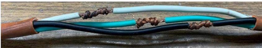
Repeat for the white and green wires. If necessary, pull on the two cables to take up any slack.
