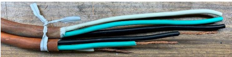
I then took a bag tie and secured the two ends together with the ends of their sheaths lined up.
