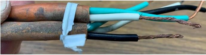
And, finally, I cut and stripped the black wire to match the white wire. I just noticed that the white wire's conductor is a little longer than the black wire, but that is OK.
