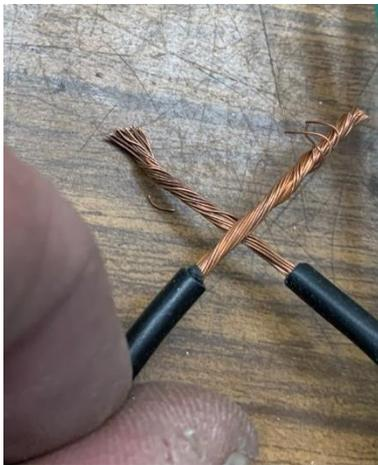
Cross the black wires about  $\frac{1}{4}$ -inch from the insulation. Then wrap each wire around the other. This forms a [Western Union](#).
