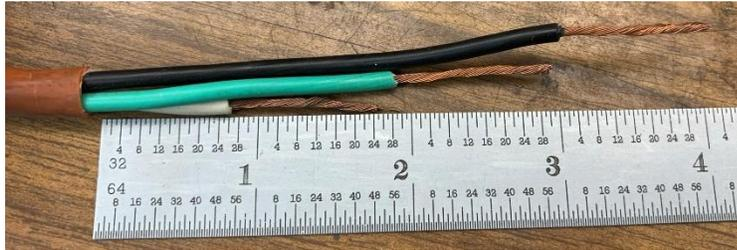
I then stripped 1-inch of insulation from the end of the black wire. The green wire was trimmed to 3-inches long and 1-inch of insulation was removed from it. And finally, the white wire was trimmed to 2-inches long and 1-inch of insulation from removed from it.
