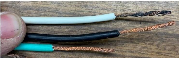
Using the black wire as a guide, I cut and stripped the white wire to match.
