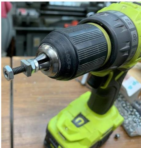
My solution was to chuck up a length of 10-24 rod in my battery powered, variable speed drill.
