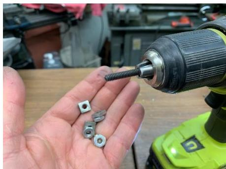
I pick up a handful of nuts and place them, one at a time, against the end of the *slowly* turning rod. If it freely engages, I run the nut all the way in. If it catches, I manually turn the nut backwards about  $\frac{1}{4}$  turn and place it aside.
