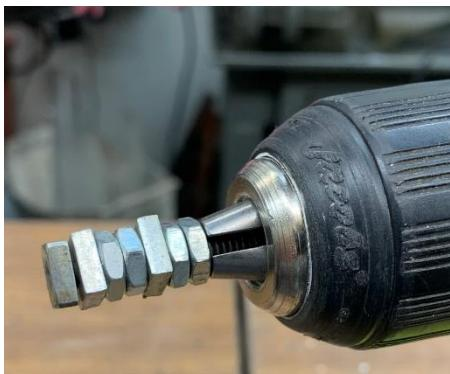
When the rod is full of tested nuts, I hold the group and reverse the drill. This spins them all into my hand.
