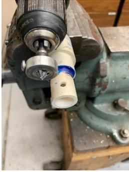
Chuck up the countersink. Drill down until the top of the countersunk hole is a little over  $\frac{1}{4}$ -inch in diameter.
