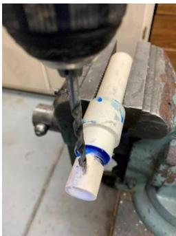
Chuck up the #7 drill and carefully drill through the PVC pipe wall. Go slow, so you do not cut the other side as you break through.
