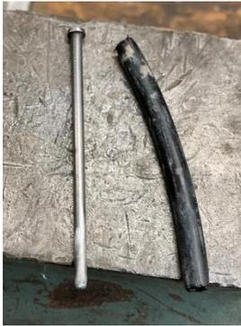
Cut a length of spaghetti line approximately equal to the length of the mandrel. The mandrel must be a loose fit to the inside diameter of the line.
