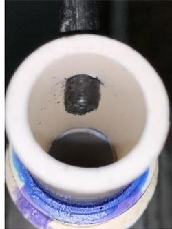
There is a small amount of damage to the outside diameter of the line, but it is a tight fit and will not leak.
