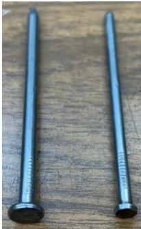
I took a 10 penny 3-inch long nail and ground the point off. The end was then rounded. The head was turned down to around 0.2-inches on my lathe. You can free-hand grind it with no loss of functionality. This will be our mandrel.
