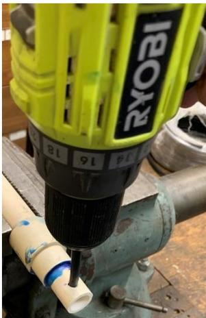
Firmly push down on the drill while the end of the spaghetti line is seated in the countersunk hole. Then run the drill at the lowest possible RPM. You will feel the assembly feeding in. When about  $\frac{1}{4}$ -inch of the line has penetrated, you are done.
