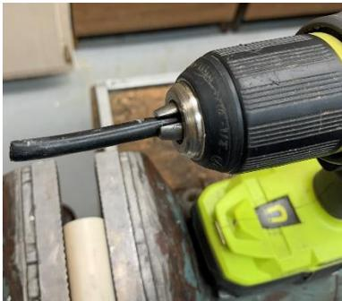
Chuck up the spaghetti line with its mandrel with the head inside the chuck. Tighten the chuck until it firmly holds the assembly. Too tight, and the chuck will damage the line.
