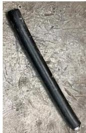
Notice that the spaghetti line is supported by the mandrel. There is room for the line to compress as it goes through the hole in the PVC pipe.
