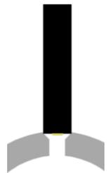
Do not run the drill too fast as this will machine away the outside diameter of the line and cause it to leak.
