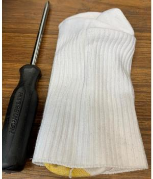
Invert the end of the sock and pull the toe through such that the overall length of the pocket is about 1 inch less than the length of the screwdriver.
