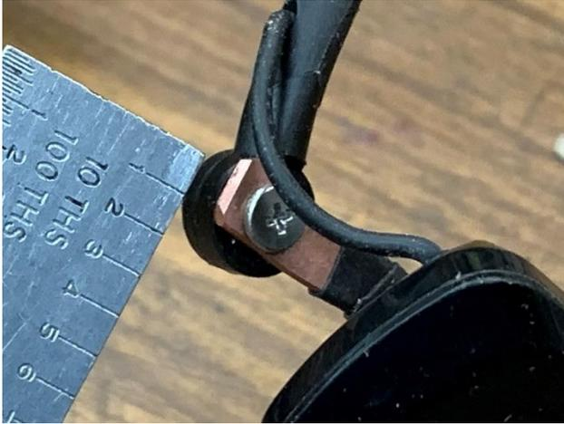
I smashed the end of the wire with a hammer and cut it square. Next, I drilled a hole, by eye, that would pass the tiny screw used to secure the original part. Then I cut it to the final length.
