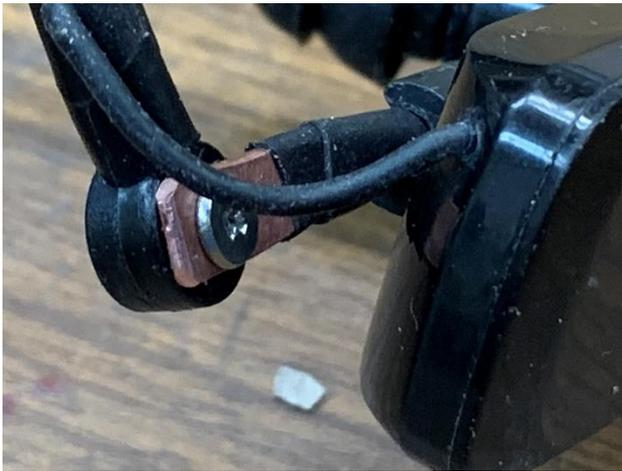
I sleeved the copper with two layers of shrink tubing. After heating, I used my hammer to slightly flair the end. This keeps the shrink tubing from sliding off.
