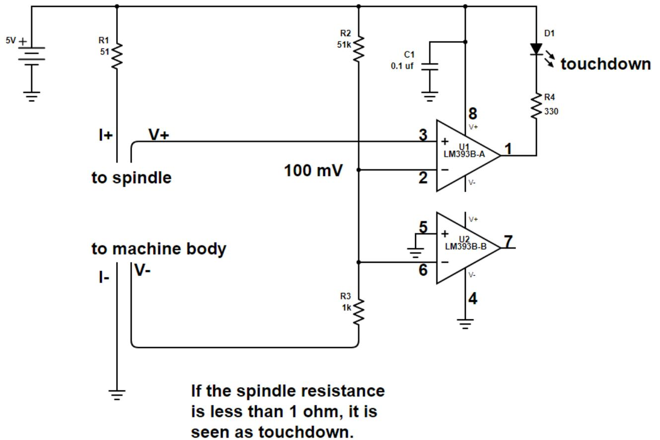
To maintain the same LED brightness, I have reduced the value of R4. I removed R5 because Probe detect is not needed.
