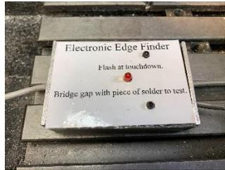
The bottom of the enclosure, which rests on the mill table or lathe ways, provides the machine body's electrical connections. Two magnets inside the enclosure ensure good electrical contact is made with the table or ways.
