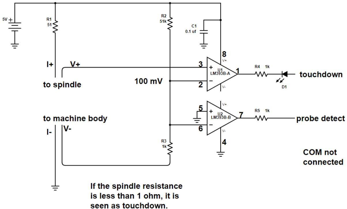
The Kelvin Connection, described on page 5, consists of I+, I-, V+, and V-. A poor connection here will cause a false reading.
