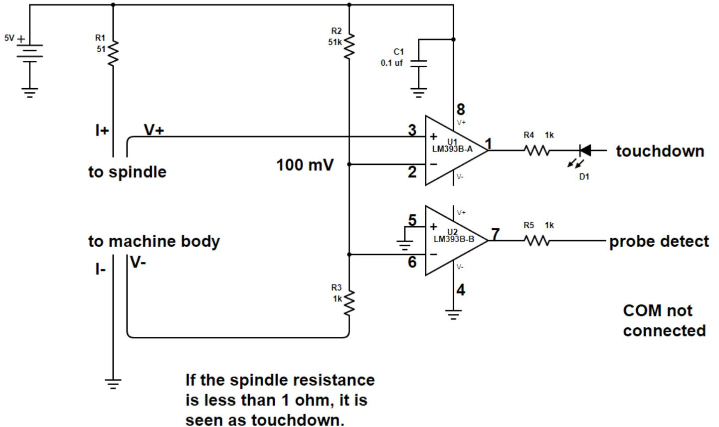
R1 continuously dissipates 1/2 watt, so I have specified a rating of 1 watt. R2 is 0.1 watts. R5 continuously dissipates 120 milliwatts, so I have specified a rating of 1/5 watts. To minimize the diversity of part types, R3, R4, and R5 are the same value and power rating.
