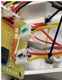
I- and V- are separate wires that run to the metal enclosure of the EEF. When this enclosure is placed on the mill table<sup>7</sup>, a low resistance connection to the machine's body is made. These four connections form the Kelvin Connection.
