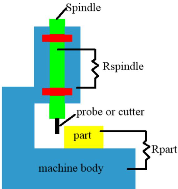
Two resistances are involved in detecting touchdown using a [non-insulated probe](#) and an Electronic Edge Finders (EEFs). The spindle resistance,  $R_{\text{spindle}}$ , is the total electrical resistance inside the two spindle bearings. It varies from many ohms down to almost zero. The part resistance,  $R_{\text{part}}$ , ranges from about 0.05 ohms to nearly zero<sup>6</sup>. They are read by measuring the resistance between the spindle and the machine body.
