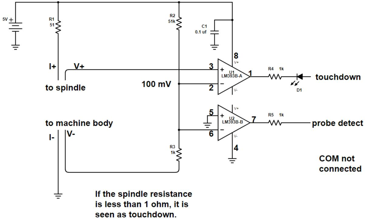
The test current is  $\frac{5V}{R_x+R1}$  where  $R_x$  is the unknown resistance. This large current causes a voltage drop in the wires associated with  $I+$  and  $I-$ . This voltage drop is small compared to 5V, so it has a minimal effect on the test current.
