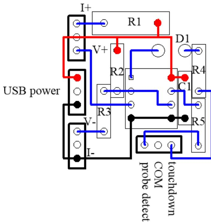
I have assumed all through-hole devices and connectors. The board is 1.2" by 1.2".
