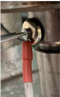
Two wires, I+ and V+, run to the magnetic clip that holds onto the spindle.
