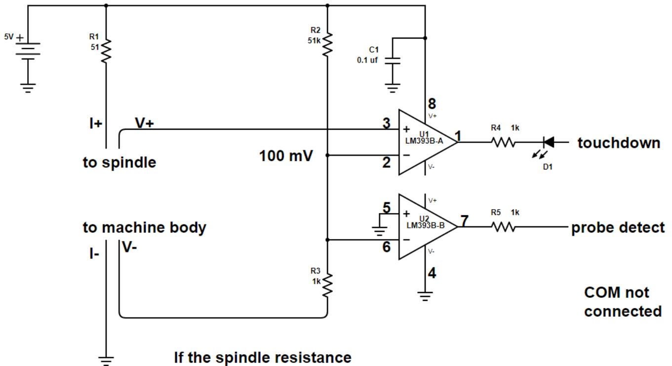
If the spindle resistance is less than 1 ohm, it is seen as touchdown.
