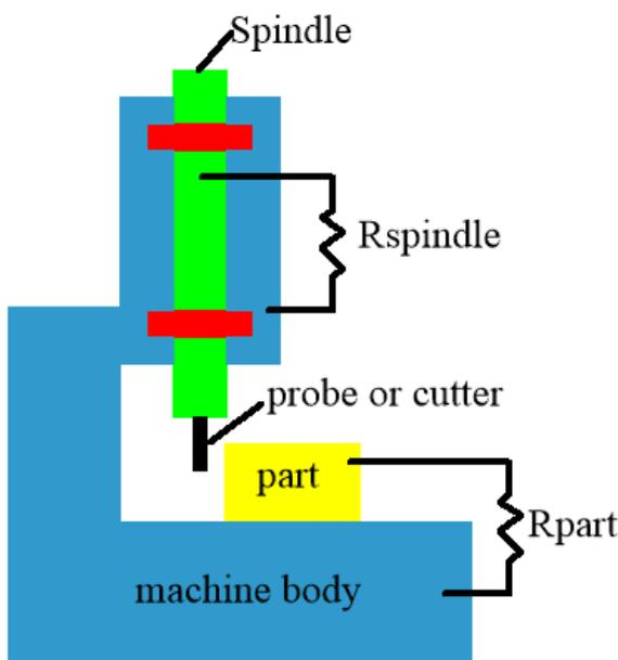
With the EEF’s enclosure sitting on the machine body, my magnetic probe can have no more than 5V on it. When connected, it is typically less than 0.2V. Then a current of less than 0.1 amps flows through the bearings.
