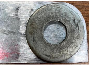
You can see that the finished radius is a close match to the "filing button" and I didn't have to drill a mounting hole.
