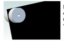
Real filing buttons are hardened cylinders with a hole in the center. They come in pairs and are bolted through the stock near a corner. Then you file down to the button and get a very precise rounded result.
