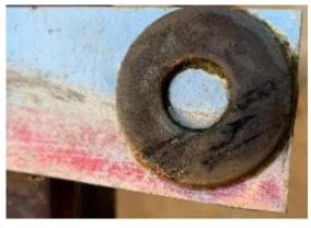
I then flipped over the washer onto the stock and quickly heated it and the stock with a torch<sup>2</sup>. It is easy to adjust while hot. When satisfied with its location, I sprayed the washer and stock with water.
