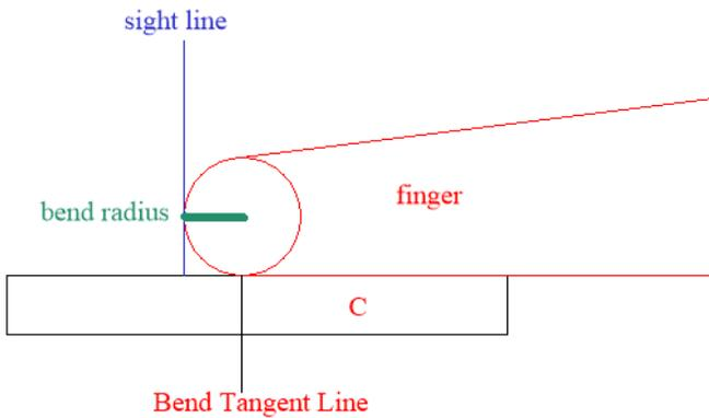
With the **C** area under the finger, I want to form the bending radius, which starts at its bend tangent line. That's nice, but I can't see the BTL since it is under the finger.
