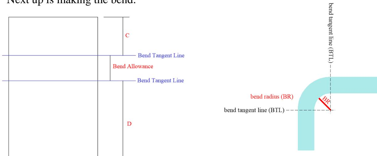
The material used in the bend is bounded by the bend tangent lines (BTL).
