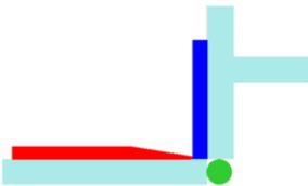
3. Set the fingers (in red), so when the apron is set vertically, the material to be bent (in dark blue) is a tight fit against the end of the finger.
