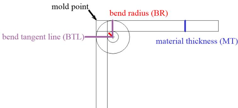
The set back (SB) is the distance from the mold point to the start of the bend, the bend tangent line (BTL).
