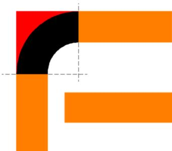
A sharp 90° bend means that the material must go all the way to the corner while the radius bend “cheats” the corner. Therefore, we use less material in the radiused bend than in the sharp corner.
