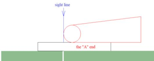
Slide the "A" end of the stock under the fingers. Sight straight down at the end of the finger and adjust the stock, so the sight line is just visible. Clamp down the fingers and make the bend.
