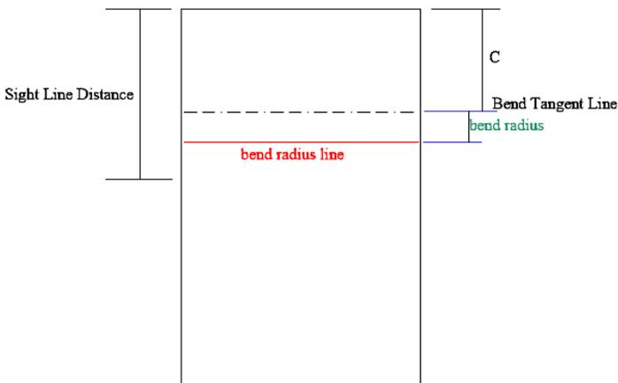
I can make a new line that is offset by the bend radius. Call this the **bend radius line**.
