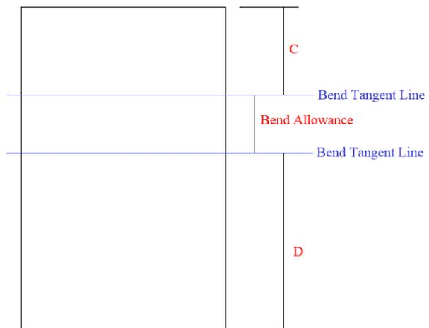
With C and D established, we replace the set back and mold point lines with the Bend Allowance. Call the lines above and below the bend allowance **bend tangent lines**.
