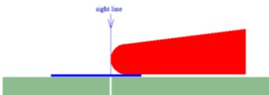
7. Slide the short end of the strip under the finger of the brake such that the line barely shows. Clamp the finger and bend 90°. Repeat on the other end so that a “U” is formed.
