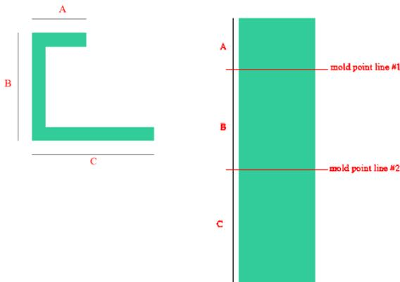
With two bends, there are three distances, A, B, and C, to the two mold point lines.
