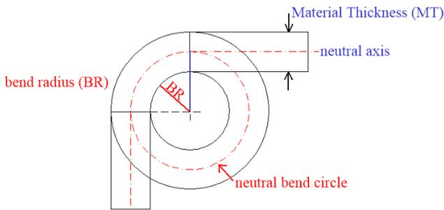
The bend allowance (BA) is  $\frac{1}{4}$  of the circumference of the **neutral bend circle**. If the neutral axis was at the centerline (i.e.,  $\frac{1}{2}$  of the material thickness), the circumference (C) would be:
