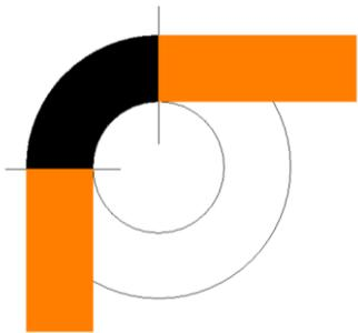
A practical bend includes a radius. If you tried to make a sharp 90° bend, the metal would likely crack.
