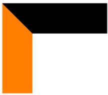
If you could make a sharp 90° bend, no material would be used in the bend.
