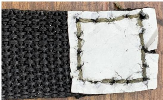
After sewing, the paper guide is partially torn by the thread as we saw in Nelson's suggestion. This makes it easier to remove.
