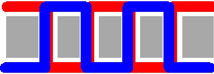
In Nelson's stitch, the thread bends at the holes in the material. As force is applied, the holes will elongate, and the bend of the thread will be gradual. This distributes the force, so the thread is less likely to break.
