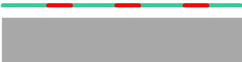
Nelson's second suggestion related to marking the path and location of the holes. He marks up a piece of paper and staples it to the material. The green line represents the line on the paper while the red dashes are the marks for the holes.
