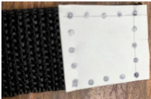
All needle locations have been marked with the stamp. In hindsight, I should have drawn lines on all four sides. The dot on the lower-left corner is the overlap of two stampings, and they did not perfectly align.
