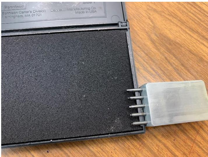
The plastic fork does work, but the tines easily bend. I made a replacement using a block of aluminum and some 4 penny finishing nails. The nails were first press-fit into the holes. Then I snipped them approximately to the same length. The belt sander finished the alignment.
