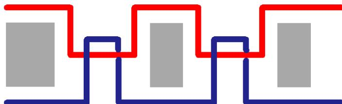
With the lock stitch, this force is concentrated at the point where the two threads lock together.
