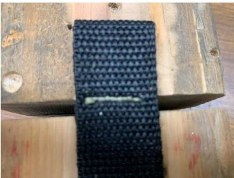
I line up the point of the needle on the material and push the awl straight down. No drama, no blood. The wood flanking the gap provides good support for the fabric.
