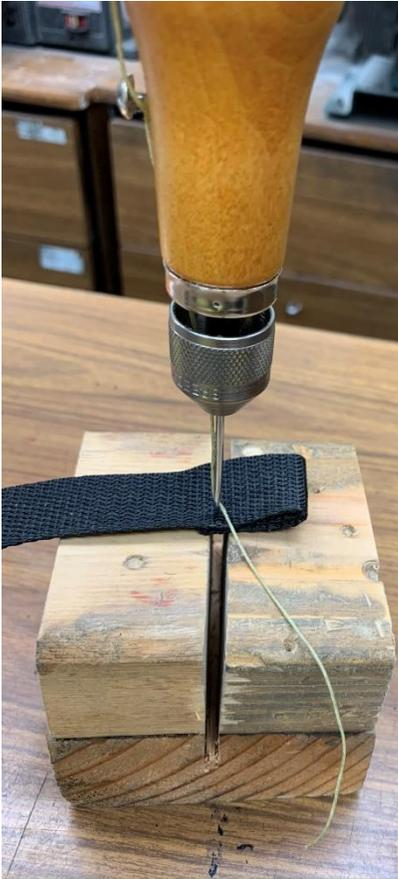
Both of these problems are solved by making this “sewing block.” I made it by gluing two pieces of 2 by 4’s to a third block. The gap is around 1/8-inch. I then sawed down a little more so
