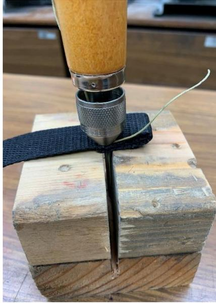
the collet would hit the material before the needle struck wood. I want to protect my flesh and the needle from damage.
