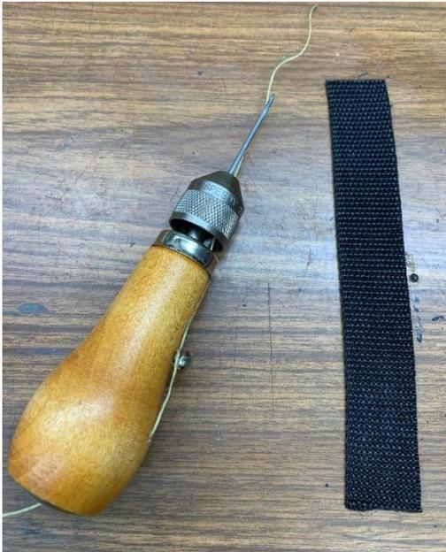
My Speedy Stitcher is perfect for sewing woven straps and heavy material. The needle is sharp, and the handle gives me plenty of area to push down hard. I can go through just about any soft material.
