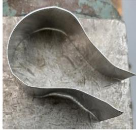
Then, I place the warm plastic patch around the piece of scrap pipe and apply even pressure by pulling on the ends of the piece of sheet metal. The goal is to form the patch to be a tight fit to the outside diameter of the pipe.
