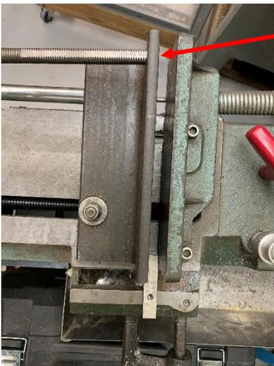
My favorite solution is to add a jack screw to the far end of the movable jaw. This can be adjusted to any depth in moments.
