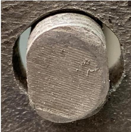
Rotate the screw 90° and the threads engage.
