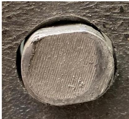
In the unlocked position, the screw's flats are horizontal. This disengages the threads and permits sliding in and out.
