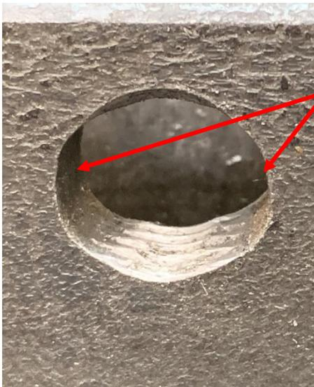
The hole in the movable jaw is first drilled and tapped to match the screw. A round file is used to remove the threads on the sides.
