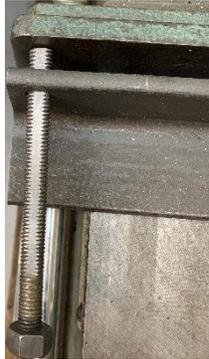
To use, I feed the screw in until it touches the fixed jaw. Then turn the screw until it is snug.
