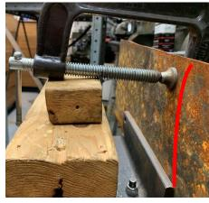
As I tighten the clamp, it will tend to become perpendicular to the thin stock. However, since the threaded part of the clamp is resting on the wood block, the top of the stock is forced to bend slightly to the right.
