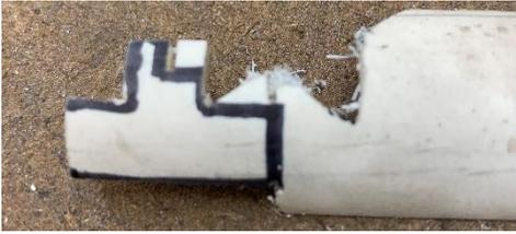
Here is where I went freeform. Ultimately, I wanted to be able to cut the top horizontal lines but the saw blade needed some room. By going in at an angle, I can clear out material.
