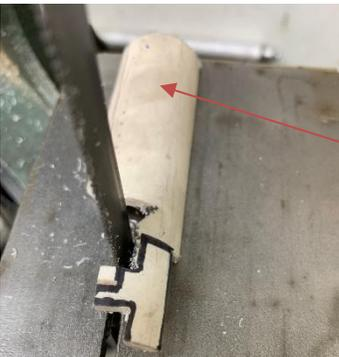
But I wasn't that smart so I made a few wasted cuts before I could get the blade in the right orientation. Note that my "handle" is now behind the blade. A bit awkward to hold but far safer than trying to grasp the part from the front.
