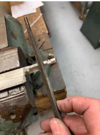
The stock was then clamped in my vise with the attached part sticking out. I used a file to bring the part to final size.
