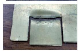
After bending the tab a few times, it broke off. Notice that the break was on the scrap side of the layout line which is certainly a good thing. You can see distortion of the metal on the other side of the line, a bad thing. A few whacks with a hammer should flatten it out. Then a file will remove the remaining metal down to the line.
