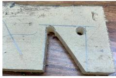
Sawed one flank and the diagonal. Forgot to saw the other flank but that will be done later.
