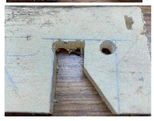
The slivers were broken out with a screwdriver.
