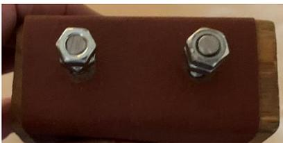
I punched holes in the belt to permit the screws to pass through. The smaller block was drilled with a #7 drill and went through to the surface of the larger block. Then I drilled ¼-inch holes in the larger block about 1-inch deep. Before assembling, I placed a ¼-inch ball bearing in each hole, which made turning the screws easier. When I turned in the screws, they cut their own threads in the smaller block.
