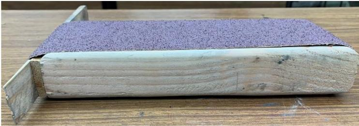
When the belt stopped stretching, I cut the thin end of the shim off.
