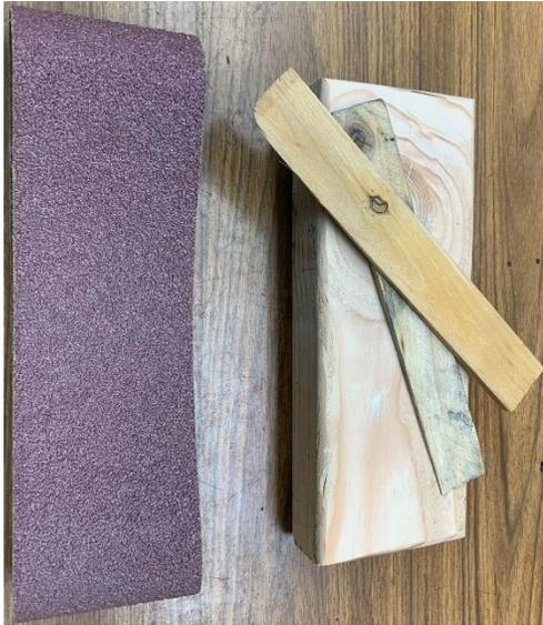
This tool also uses a 2 by 4 block. I calculated its length from the size of the 3-inch wide belt. Take the circumference and subtract 3-inches. Then divide by 2. For example, for a 21-inch belt, I first subtract 3 to get 18. Then I divide by 2 to get 9-inches.
