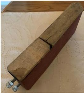
My first attempt at duplicating the sanding block involved two blocks of 2 by 4's and tensioning screws. The screws jack the blocks apart.
