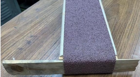
The slack reduced as I slid the second shim into position. The base of the shim faced the belt.
