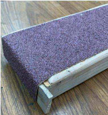
The fat end of the shim was cut such that about ½-inch stuck out. This permits me to tighten the belt a bit more and also gives me something to grab when I need to remove the shim.
