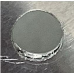
Since the sheet metal was well supported by the tool, there was no distortion around the hole.
