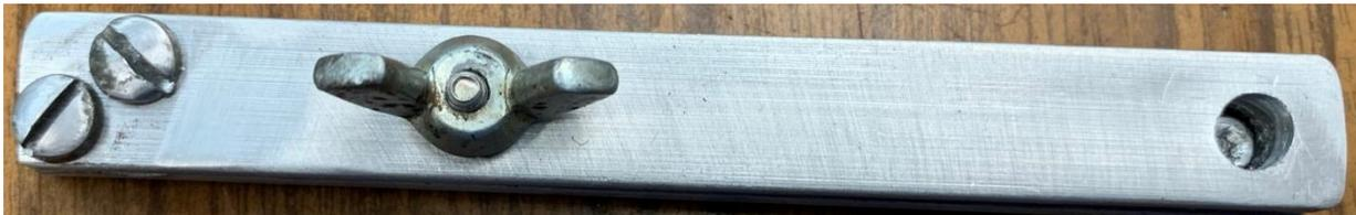
I first drilled through both bars with my #32 drill. Then I ran my #27 drill through the top bar. And, finally, I ran my 6-32 tap through the bottom bar.
