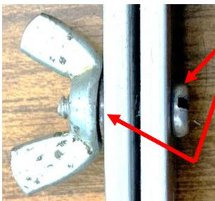
These threads, cut into aluminum, are not robust, so I ran a steel screw in from the back. On the top side, I put down a small steel washer and my wing nut. In this way, I have steel on steel for minimum wear. If I ran a screw in from the top, I would have the steel screw wearing on aluminum threads. That wouldn't last long.
