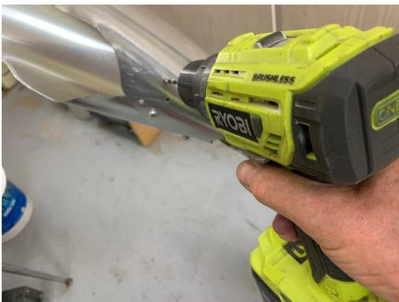
As I start drilling, the drill tends to dance away from my black dot. I also bend the soft aluminum sheet metal. By pushing harder plus backing up the site with my hand, the dancing stops along with the distortion. Hmmm. What's wrong with this picture?
