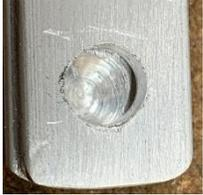
The guide hole was drilled all the way through the top strap and deep enough into the bottom strap to contain the point of the drill.
