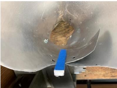
The tool clamps the inside curl of sheet metal. This guarantees that the hole through the exterior sheet metal will align with the inside.
