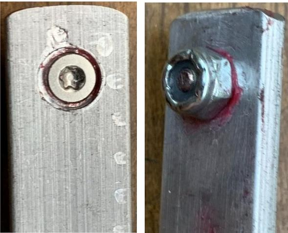
I coated the #4 screw with synthetic grease and put a Nyloc nut on the back. The screw freely turns.
