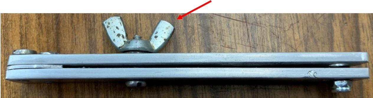
I give the wing nut a half-turn, and the top and bottom bars squeeze together.
