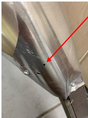
This black dot is where I want to drill a 10-32 clearance hole. Since the hole goes through two layers and is curled around a frame, removing the stock and placing it on a flat surface for drilling is not practical.
