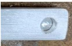
The final step was to use my 10-32 clearance drill to partially drill through the back strap. This enables the drill to cut entirely through the sheet metal without going into my hand.
