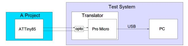
The Translator accepts a nonstandard signal from the ATtiny85 and converts it to bytes. These bytes are sent out the USB, where they are displayed on the PC.
