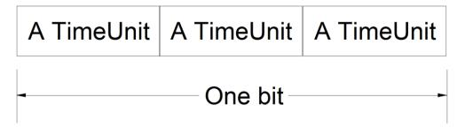
The second timing constant is TimeUnitMicroS. It is approximately the width of a TimeUnit, although another 200 microseconds are added to it as the code executes. If the bytes you are sending from the ATtiny85 are being corrupted, try increasing this time. Just remember, there are 6 TimeUnits in the Header plus 24 TimeUnits in the byte, so increasing this constant by 100 microseconds means it will take 3000 microseconds *more* to transmit it. See page 14 for more detail.
