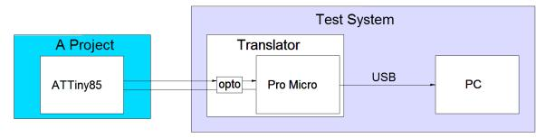
The embedded ATtiny85 drives one, user-specified, IO pin. This signal feeds into my Test System. The Test System consists of a Translator and a PC running a Terminal Emulator.
