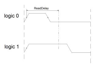
Right after the receiving logic determines the TimeUnit, it multiplies by 1.5 and calls it the ReadDelay.
