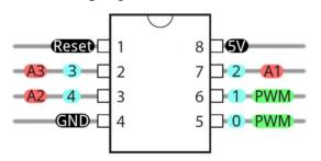
Can't have it all! With such a small package, there are only 5 easily usable Input/Output (IO) pins. A sixth pin can be configured to be a "weak" IO pin, but then you give up the ability to reset the device.
