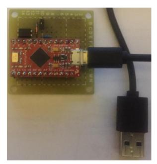
The USB connector on the Pro Micro is delicate. If you have a spare cable, plug it in permanent.
