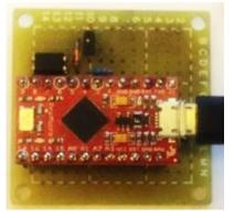
The Translator consists of an optoisolator and a Pro Micro. The optoisolator permits me to run the ATtiny85 and my Test System on different grounds, plus protects the PC from possible ground fault currents generated by my project<sup>4</sup>.
