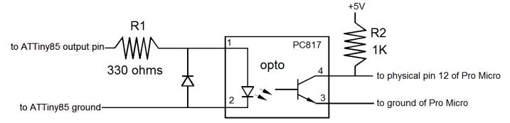
This little circuit could prevent you from having a very bad day. Ground from your laptop or PC connects on the right. Ground on the ATtiny85 connects on the left. If, for some reason, these two grounds are not at the same voltage, an unknown and potentially destructive current can flow.
