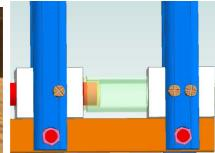
In one action, I push each pair of arms together while moving the pairs of arms towards each other. This rendering includes an x-ray view of the hard pipe and coupler.
