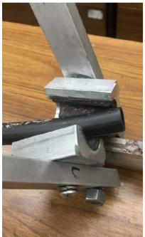
The soft pipe is placed inside the rubber lined jaws while
