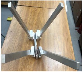
In the load position, the two sets of jaws open to accept the soft and hard lines.
