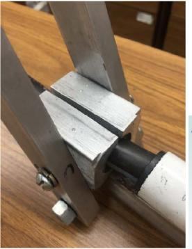
Closing each pair of arms secures the jaws around the pipes. The end of the soft pipe is touching the opening of the compression sleeve inside the PVC coupler.
