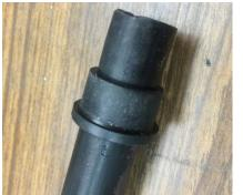
Many couplers exist that connect soft pipe to hard pipe. The most cost effective design is a compression sleeve. I paid 2.50 for a bag of  $5^3$ . The fancy couplers are over 4 each.
