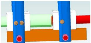
Attach the jaws with <sup>3</sup>/<sub>4</sub>" long <sup>1</sup>/<sub>4</sub>-20 screws. The soft jaw screws are Loctite'd in place such that the jaws can smoothly pivot. The PVC jaws use the same screws plus lock washers.
