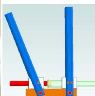
The soft pipe jaws slide on the connecting bar. These jaws are free to pivot relative to their arms. This forces these jaws to stay in alignment with the hard pipe.
