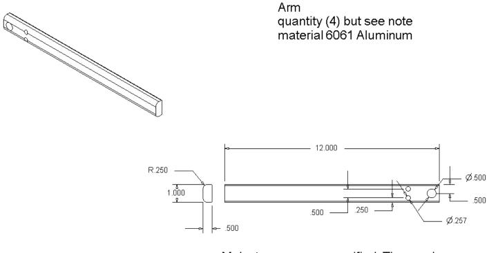
Make two arms as specified. Then make one arm as specified but with only the top 0.257" hole. The forth arm is with only the bottom 0.257" hole.
