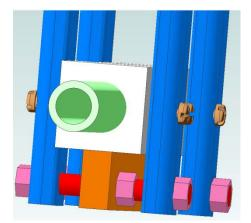
Thead the rod half way through the linkage bars and secure with a nut on one side. Attach the arms and put nylon lined locking nuts on the outside.
