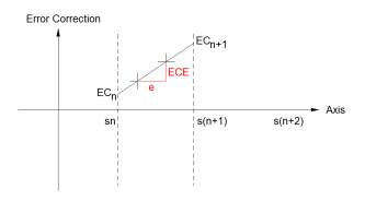
Our Home sensor has an error of  $\pm e$  which causes an Error Correction Error (ECE). The software assumes we are at a given location along the axis but due to e, we are actually shifted over. This shift in location causes the software to generate an Error Correction that is also shifted.
