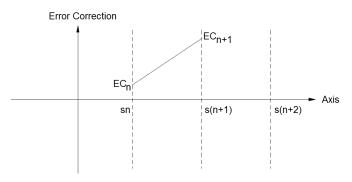
The Centroid Screw Mapping table for each axis consists of data taken at 0.5000 inch intervals. This data is collected while moving away from Home and also towards Home. The physical location of Home on a given axis is set by a Home sensor.
