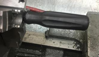
Each screwdriver went into my lathe for drilling.
