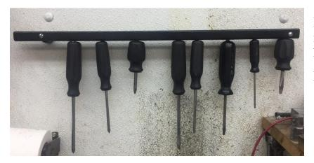
I installed a neodymium magnet<sup>2</sup> into the top of the handle of each screwdriver. A dab of 5 minute epoxy did the trick.
