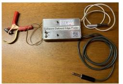
My Software Defined Edge Finder (**SDEF**) has a repeatability better than  $\pm 0.0001$  inches. The cost of the electronics is estimated at under \$10. This device is compatible with Centroid's Computer Numerical Control's automatic touchdown feature.
