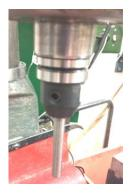
The electrical resistance between the spindle and the rest of the machine must be at least 0.1 ohms.
