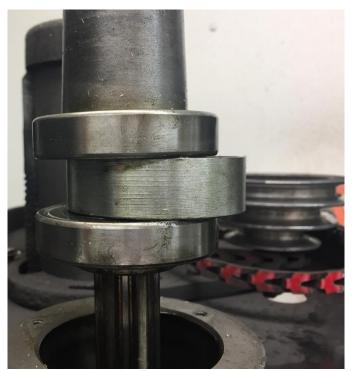
Here you see the drive bearing assembly pulled up exposing the two bearings and spacer ring. I have pushed the ring off center to make it more obvious.
