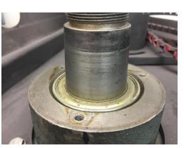
You now see the top sealed bearing. The bearings are a snug sliding fit in the casting.
