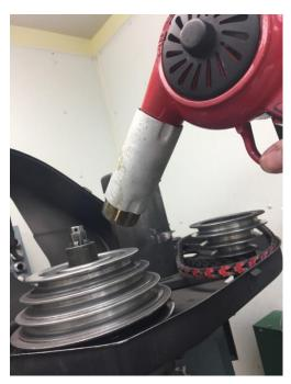
Using a heat gun, I warmed the pulley for about 2 minutes. An audible click can be heard as the pulley lets go of the taper. Warning: do not use a torch for this operation. It can damage the bearings and possibly warp the pulley.
