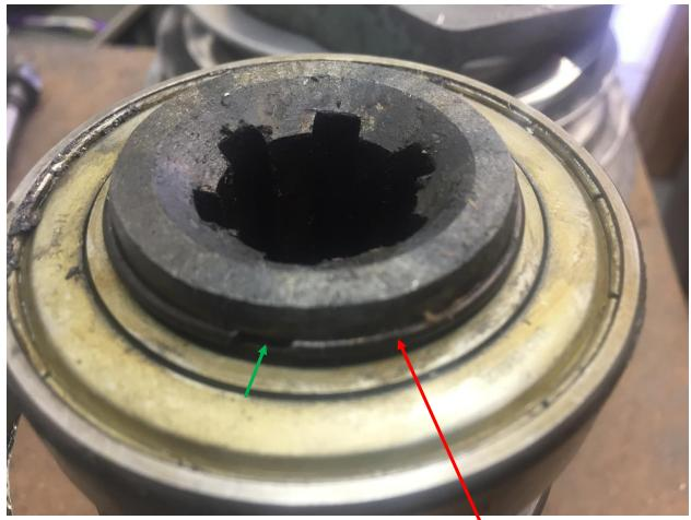
The bottom of the spindle drive bearing assembly has a clip which prevents the lower bearing from sliding off. I used a thin blade screwdriver in the gap (green arrow) to lift this clip out.
