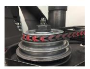
This pulley is secured to a hollow shaft which has an internal spline.
