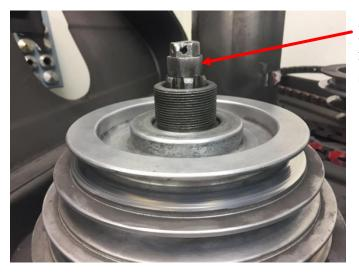
I have a draw bar of my own design and it must be removed because it blocks the spline from sliding all the way down.
