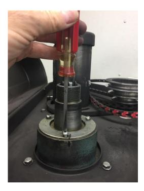
Remove the three screws and cover ring.
