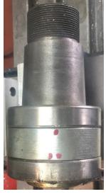
I call the pulley, hollow shaft, and its bearings the "spindle drive bearing assembly".
