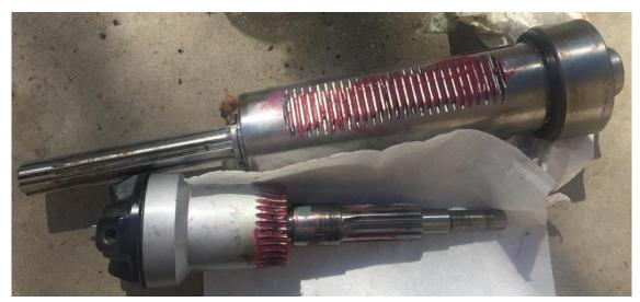
Before installing back into the head, I greased up the rack, pinion gear, and drive gear.
