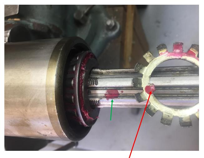
Before sliding off the tab washer, I degreased the inner tab and the spline it engaged (green arrow).
