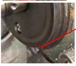
During installation, you loosely tighten the knob, wind up the spring by turning the cylinder (clockwise?), and lock it in position by engaging fingers in the head and cylinder base. Then finish tightening the knob.
