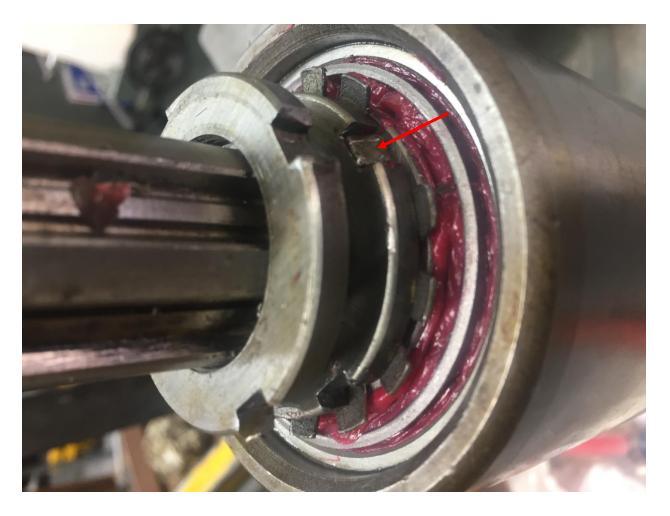
The inner nut is held in place with a tab washer. There are 3 notches in the nut, and there are many tabs on this washer. One of these tabs will align with one of the notches to prevent rotation.
