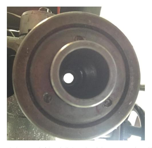
The bottom end of the spindle has a threaded grease cap. Using a drift and a small hammer, you can get this ring to turn. It is a right-hand thread.
