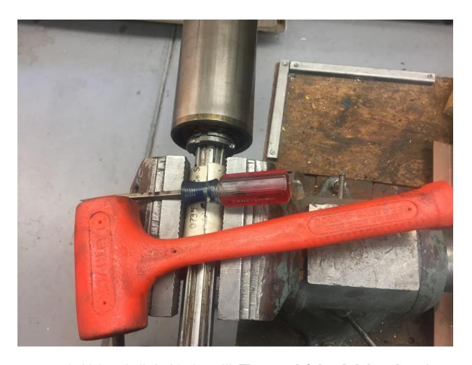
Two nuts hold the spindle inside the quill. **These are left-handed threads**. Using a screwdriver and dead blow hammer, I gently unscrewed the outer nut.
