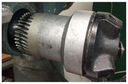
slide the pinion gear assembly into place.
