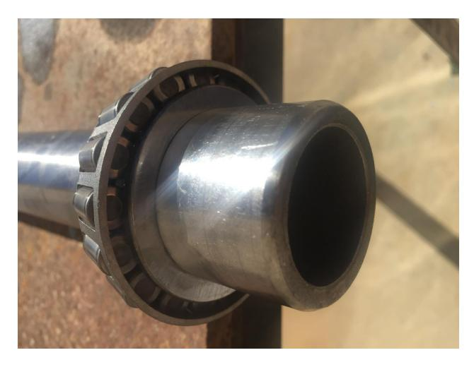
With the upper bearing removed, the quill slid out to expose the lower bearing. I degreased this bearing in place. It was placed down in a can of degreaser for 15 minutes. Then I soaked it in "Simply Green" to remove a few stubborn bits of grease plus remove the degreaser.
