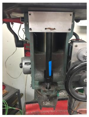
The black cylinder is a gas piston that removes backlash from my Z-axis. By lowering the quill and loosening a screw supporting the bottom of the piston, I was able to release the pressure.
