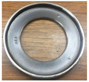
Here is the inside of the grease cup after being degreased.
