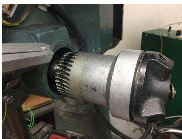
With the quill supported by the blocks of wood, pull the horizontal shaft out.
