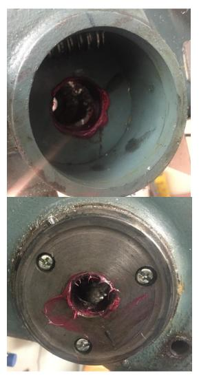
I put some grease in the holes that support the pinion gear assembly.
