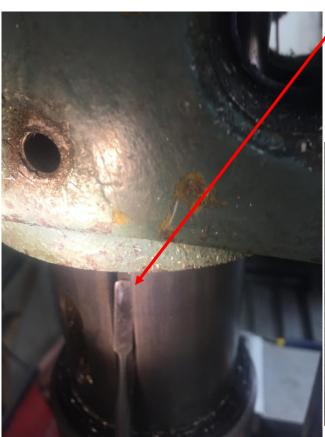
Slide in the anti-rotation block with the curved end pointing down. Sight through the threaded hole and position the block, so the hole in its face is aligned.
