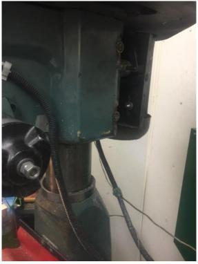
Raise the head up to the top of the column. This makes room for the quill to come out the bottom.
