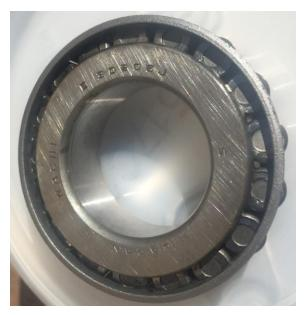
Here is the upper bearing degreased and ready to be repacked.
