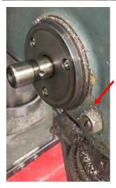
Below and to the right of the spring cylinder is the anti-rotation stop. Insert a screwdriver into the slot and turn the nut counterclockwise to release. Then back out the threaded rod.
