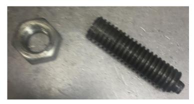
The nub on the end of the threaded rod engages a small block. This block rides in the quill's anti-rotation slot.
