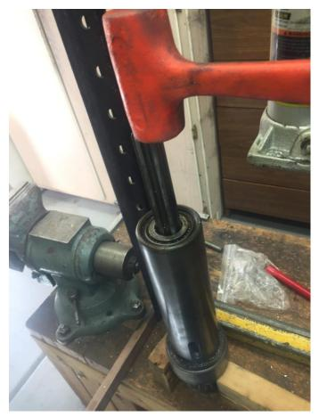
With both nuts removed, a light tap with the dead blow hammer was enough to move the upper bearing. Notice that the bottom of the quill was supported on wood blocks to permit the lower bearing and spindle to drop down.
