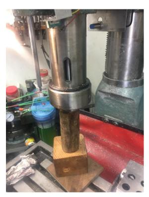
Lift up on the quill, remove the blocks of wood, and carefully lower the quill/spindle assembly down.
