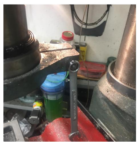
Loosen the bolt on the back of the lower spindle bearing clamp. You may need to pry the gap open a little, but then the clamp should slide off the bottom.
