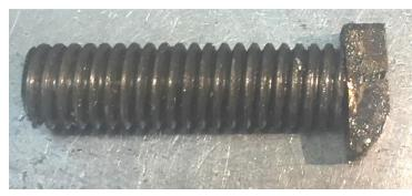
Here you see the block fitted to the end of the threaded rod. The curved end points down in the slot.
