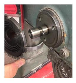
Lift off the spring assembly to expose the horizontal shaft. The other end of this shaft has the clutch.
