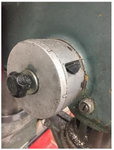
This large silver cylinder contains the take-up spring. That knob in the center secures it. Take care as you turn the knob counterclockwise to remove the cylinder. The cylinder can release from the head, and the spring suddenly release.
