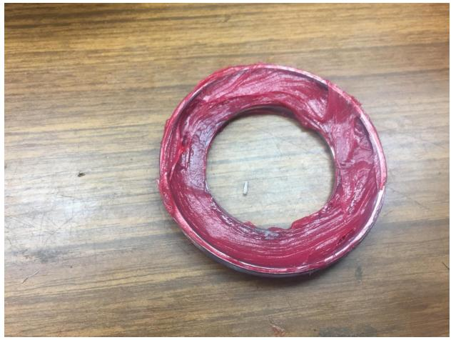
Pack the lower grease cup and screw it into the bottom of the quill. Tap with a drift and small hammer until snug.
