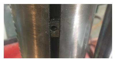
The block is a close sliding fit in the quill's slot.
