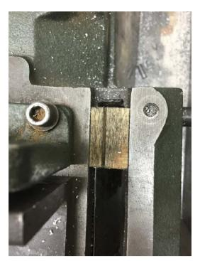
The cut line modification consists of a small block of wood. I first cut it to be a snug fit at the top of the slot that runs under the blade. Then I used the saw to make a cut about 1/8" deep. Finally, I ran my belt sander to taper the sides of the block so it would be a snug fit in the slot. I've been using this gage for a few days and it has proven to be useful. Painting it white might help give more contrast. The slot does tend to fill up with swarf.
