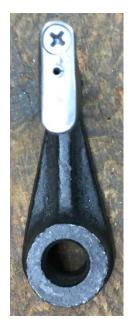
A quick trip to my scrap drawer turned up a small bit of Cold Rolled Steel<sup>2</sup>. I drilled a 6-32 tap hole first. Then I match drilled through the CRS and into the end of the stop. The CRS hole was then enlarged to a 6-32 clearance hole and countersunk to match the screw I found. The stop was tapped 6-32.
