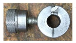
A few years ago I built this collar. On one side I cut a ¼" wide slot deep enough to accept a small magnet. The magnet is flush with the surface and glued in place.
