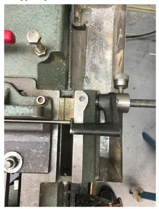
No matter that I have been using this bandsaw for many decades, I still find minor areas for improvement. Recently I was cutting some small diameter rod and realized that the built in stop did not reach it. I also realized that the only way to determine exactly where the blade would come down on the rod was to, well, bring the blade down. Not a big deal but it got me thinking about how else this could be done.
