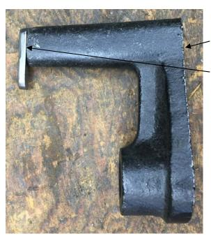
The modified stop is shown here. I first bolted the right side down on my mill table and took a light cut across the end to square it up.
