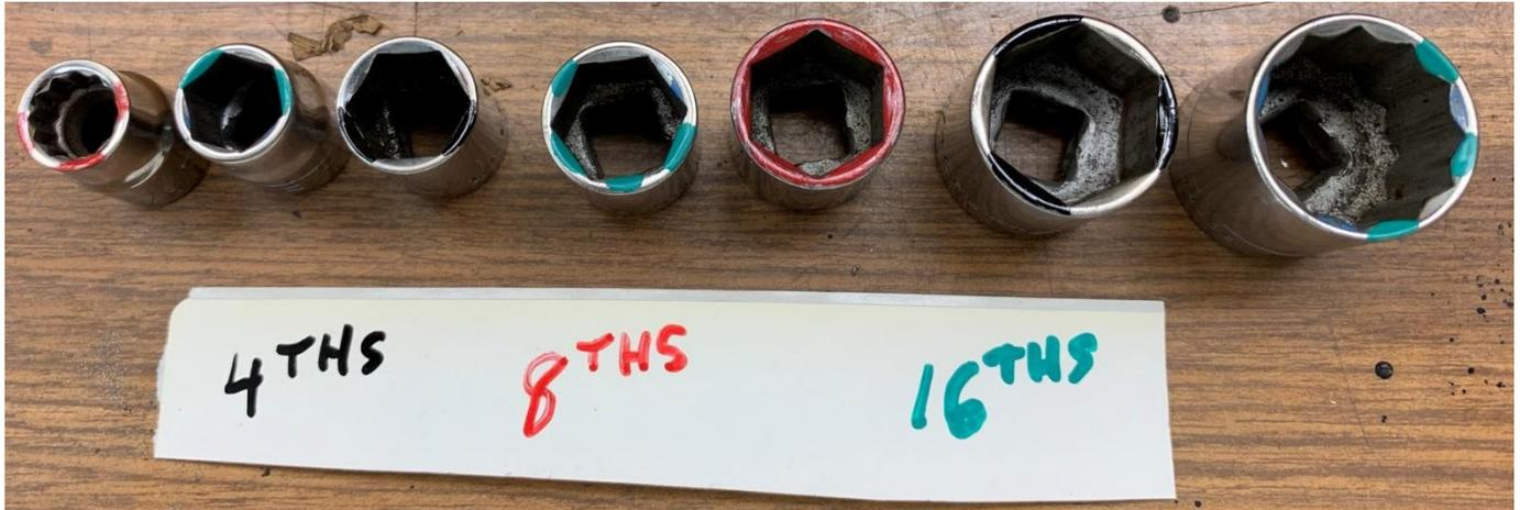
I do find that not having the color dots at 90° from each other makes it harder to find them in a glance. Compare the 3/8 socket with the 9/16 socket.
