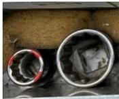
In the middle are sockets in increments of 1/8 inch. The one on the left has 3 red dots, so it is 3/8 inch. The one on the right has no dots, so it is 5/8.
