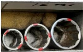
The grouping of sockets on the right is in 16<sup>ths</sup>. The smallest one has 2 dots. This could mean 2/16, but then it would be in the 1/8 inch group. Besides, it would be much smaller. So it must be 5+2 = 7 sixteenths. The middle socket has 4 dots, so this is 5+4 = 9 sixteenths. And the one on the right has one dot, so is (5 x 2) + 1 = 11 sixteenths.
