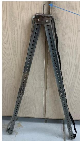
My solution was to build a bipod. A pin in the top engages a hole drilled into the mast. This prevents the bipod from sliding yet enables it to drop away as the mast is lifted vertically. The legs can be independently extended in increments of  $\frac{1}{2}$  inch.
