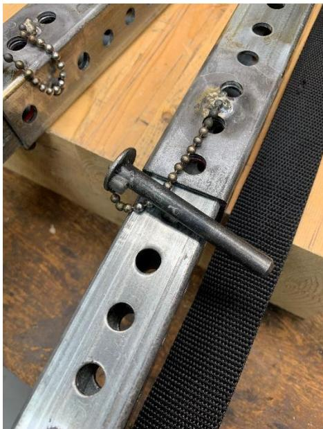
Securing each leg is a 3/8 inch diameter pin with a washer welded on top. Epoxied under the washer is a neodymium magnet that reduces the chance of the pin falling out. The ball chain is braised on. Place the pin through a hole in the larger tube and the legs are adjusted in steps of 1 inch. Place the pin through a hole in the smaller tube and the 1 inch steps are offset about  $\frac{1}{2}$  inch. In this way, each leg can be independent adjusted to the nearest  $\frac{1}{2}$  inch.
