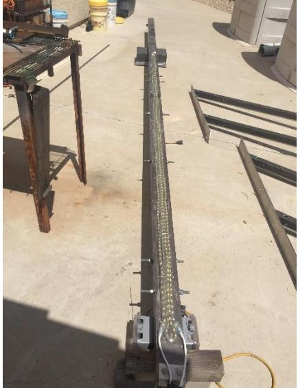
Once a year I join a team of guys that carry this mast and other parts up a mountain. This beast is 4 inches by 4 inches and 20 feet long. Although composed of 3/16 inch thick aluminum, it is heavy.
