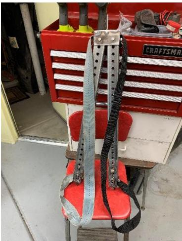
By adjusting the overall length of each leg, I am able to adjust the amount of slack in the straps. Here you see the legs fully collapsed which give the most slack.
