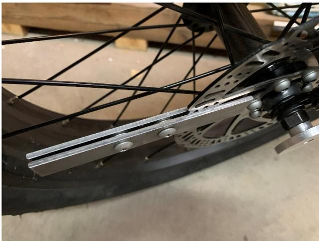
My tool is a nice sliding fit on the disc. There is plenty of mechanical advantage to gently bend the rotor true.
