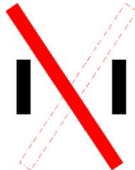
On the other hand, a problem arises if the rotor is severely bent – it wobbles as the wheel turns. The gap between rotor and brake pads will vary. The brake pads must be backed off to prevent constant dragging.
