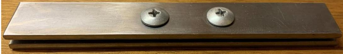
I cut a piece of 1/8-inch by 3/4 -inch strap about 4-inches long. Then I used it as a gauge to cut a second piece.
