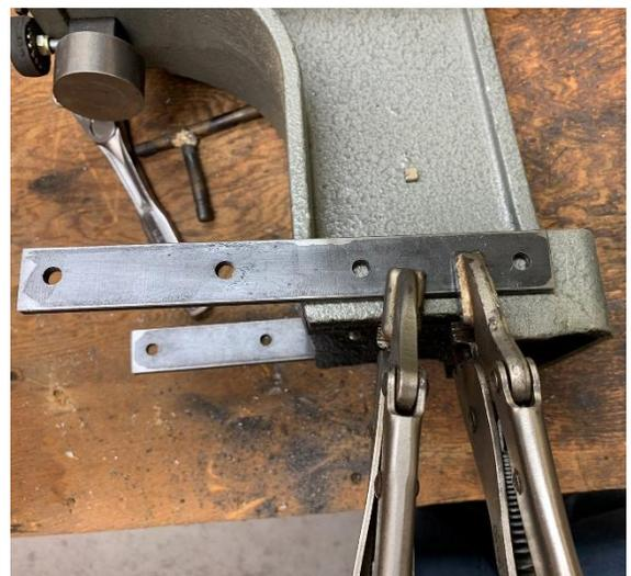
I aligned the first strap, by eye, on the rear part of the casting. Then I match-drilled the two holes using the F drill.
