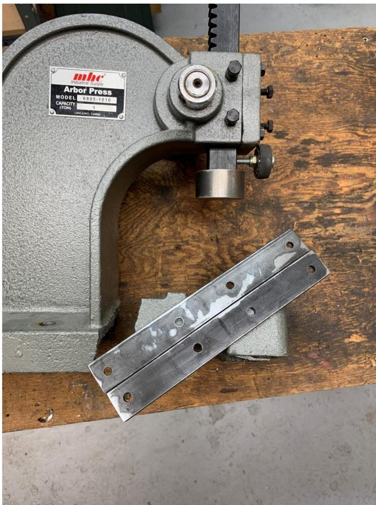
Why not try bolting on side straps? I made two from 1/8" X 1" X 8" CRS. The casting will prevent the strap from twisting, and the one inch of steel is extremely strong in shear. I selected 5/16 bolts to have about the same strength in shear.
