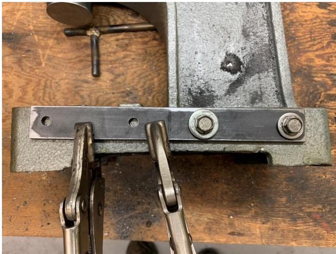
With the two casting parts pushed together, I clamped the first strap. Then I repeated the match-drill and tap process.
