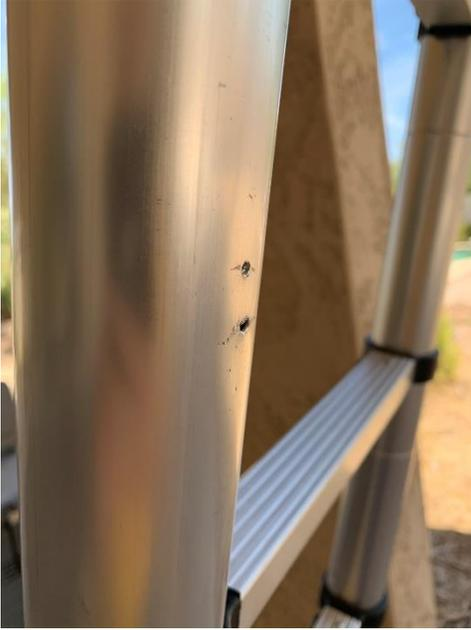
With the ladder fully extended, I drilled a 1/16<sup>th</sup> inch hole in the center of each dent. You can't see the dents here because I had low confidence that this would work, so I didn't bother to document it.
