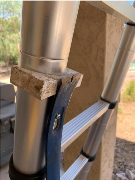
and gently pulled the dent out. I took special care to spread the force from the end of the prybar over a large area so as to not create a new dent.
