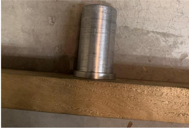
The base was built from a piece of pine with an aluminum cylinder bolted to it. This cylinder was turned on my lathe and has a diameter that is a close fit to the inside of the rod. I left a larger diameter at the bottom so the rod would not sink into the wood.
