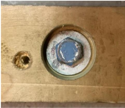
The cylinder was drilled and tapped to accept a 3/8-16 bolt. The pine was drilled out to accept a washer which spreads the load.
