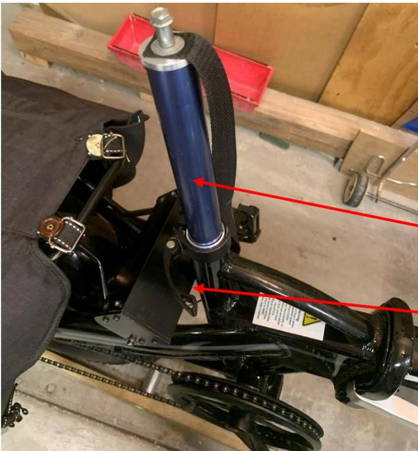
The rod is slid down the tube. It is a close sliding fit.
