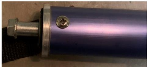
Using the same material, I turned a close-fitting plug for the top of the rod. It was drilled and tapped 1/4-20, and a shoulder bolt fitted. I drilled and tapped a hole in the side of the rod and plug 6-32, and used a small screw to secure it. The shoulder on the plug takes the force. This screw just keeps the plug from falling out during storage.
