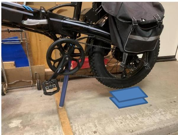
If the bike is too heavy for you to lift, place the rear wheel on something a few inches high and size the strap so it is snug when looped over the bolt. Alternately, use a Nite Ize fastener for a [rope](#) or [strap](#).
