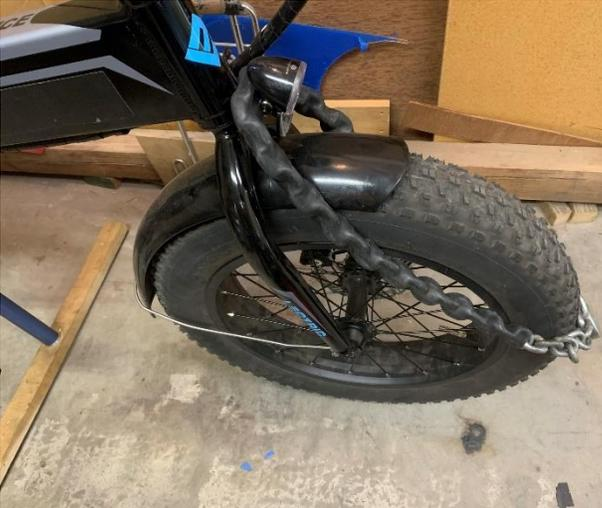
When I want to service the back wheel, I draped my bike chain and lock over the front wheel. This is enough weight to tilt the bike forward.
