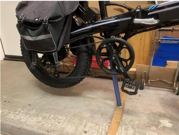
If I am working on my disk brakes or derailleur, it is best<sup>2</sup> to raise the wheel off of the ground so the wheel can freely spin. This is also handy when I'm trying to isolate an unwanted sound related to the spinning of the wheel.
