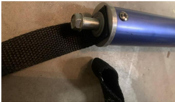
I punched a hole near the end of a piece of 1-inch wide webbing so my 1/4-20 shoulder bolt would pass through. A washer distributes the force.
