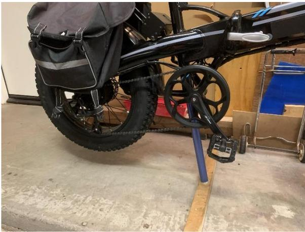
When I'm done, I again lift the bike up by the handle, unloop the strap, and lower the bike. Then I lift up the rod so I can tilt the bike back on its kickstand. And finally, I separate the base from the rod.
