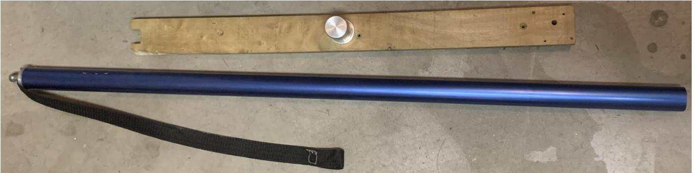
The stand consists of two parts: the base, and the rod. The rod is a hollow tube.
