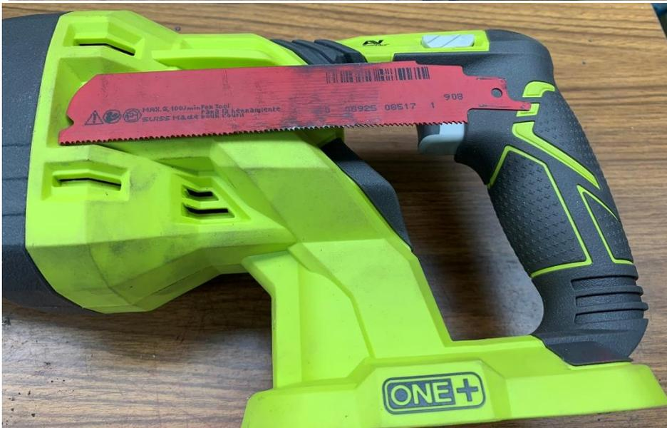
Here is the blade I expect to use most often. It nicely fits down into this pocket. I can easily peel it out of there and install the blade in the saw. If the stored blade was hit hard enough, it would fall off rather than become bent.
