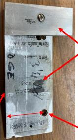
I then built a drill guide for the top hole of each 3½ inch-wide plank. It consisted of a scrap piece of aluminum angle with a plate<sup>5</sup> bolted to it. I fitted the angle to the plate and drilled through with a 6-32 tap drill. Then I opened out the hole in the angle. The securing 6-32 screw does not extend below the plate where it would hang up on the plank.
