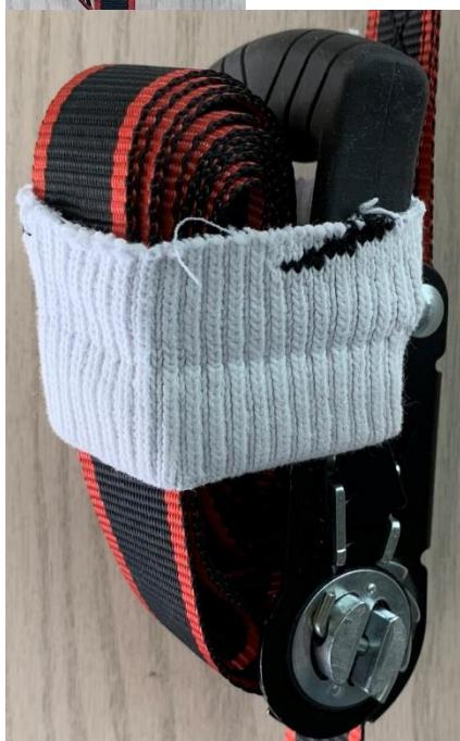
Slip the band of cut up sock around the strap and the handle of the ratchet.
