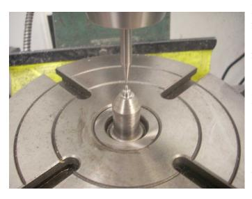
Before you can use a Rotary Table on a mill, its center of rotation must be aligned with the spindle's center of rotation. Many means exist with varying degrees of ease and accuracy. In most cases, you start with a rough alignment. My favorite method is to mount a spud in the spindle and a modified dead center in the RT's tapered hole. This can get the center of rotation of the RT to within about 0.02" of the center of rotation of the spindle. For some jobs, this is plenty good.
