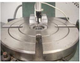
So how good was my alignment using a DRO? I put in my pin and DTI. The mill table was moved until the DTI showed I was aligned within 0.0005". I then looked at my DRO display and and saw that my X axis had been moved by 0.001". My Y axis was not moved at all. I repeated the test and this time found that no movement in the X or Y axes was needed.
