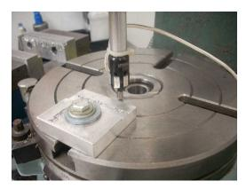
The process is repeated for the Y axis. Here you see the EEF coming in contact with the block as it has been moved to 90 degrees. At touch down, the Y axis is zeroed.
