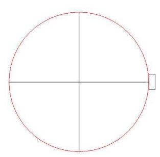
Next I crank the RT until the block is at 180 degrees. If my Y location is exactly at the center of the RT, then when I touch down on that same inner face of the block, I will be at a distance equal to the diameter of the circle inscribed by the block minus the diameter of the EEF probe. I don't care about either diameter. But if I now run the centerline function, I will see how far back to crank the X axis to end up at the center of rotation of the RT along the X axis.
