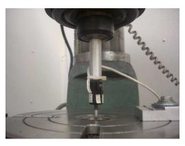
I start out with the EEF roughly centered on the RT. The tool offset is set to center.
