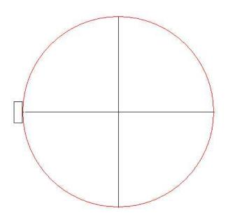
Say I attach a block to the surface of the  $RT^2$ and set the angle to 0 degrees. I then define the block's inner face as X = 0 with an Electronic Edge Finder connected to my DRO. I would do this by moving the EEF from near the center of the RT out to the block. When the EEF contacts that inner face of the block, I set my zero for the X axis.
