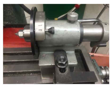
After setting up my 8 inch rotary table to be the drive for my 4th axis<sup>2</sup>, it was time to figure out the tailstock. I could buy one on eBay for around \$100 including shipping, I could make one from scratch which would take a few days, or I could adapt something I already owned. A bit of hunting turned up my 5C collet
