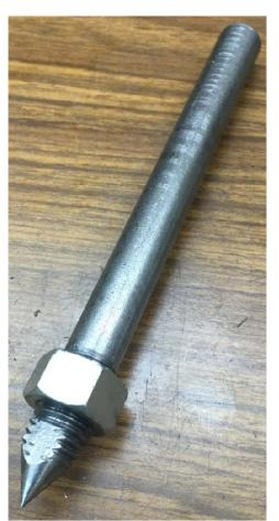
Since I wasn't sure this idea would work, I made the adjustable dead center out of ½ inch diameter CRS. I may later make one out of drill rod and harden the point.
