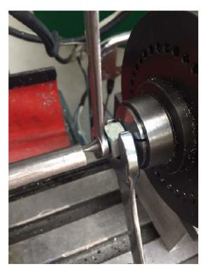
The dead center is mounted in a ½ inch collet in the spinner. I put a 5/16 inch wrench on the flats and a ¾ inch wrench on the nut. The nut is in contact with the nose of the collet. By turning the 5/16 inch wrench, I can jack out the dead center into the work piece. And finally, the collet is tightened.
