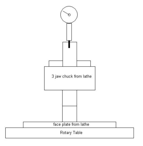
This can be done by clamping a piece of round stock, equal to the diameter of the part to be machined<sup>1</sup>, into the jaws.
