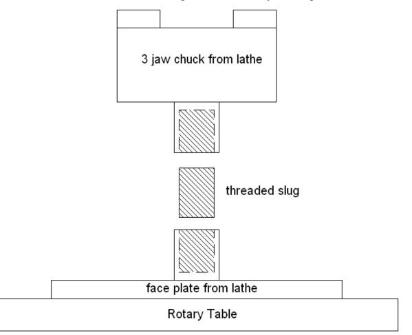
The threaded slug bottoms out in the chuck but not the face plate. The outer faces of each are able to squarely seat against each other to provide a relatively solid support.
