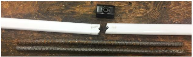
After a bit of wandering around my shop, I noticed some one foot long pieces of rebar. Nice and rough on the outside and easy to cut. It turned out they were a nice fit to go inside the broken strut. Those ribs should provide some holding power.
