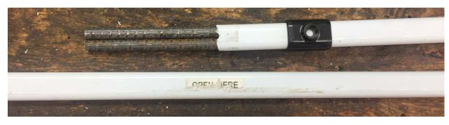
The other part of the strut had text on it so it was easy to figure out how the plastic sleeve must be positioned. I also compared it to one of the struts on the shelter. The ragged ends confirmed I had the strut oriented correctly. I didn't want to have to take this apart.
