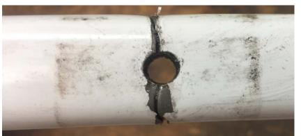
I then drilled a hole through the rebar using a sharp drill and lots of cutting oil.
