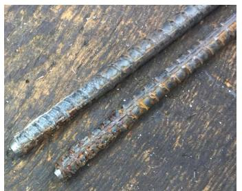
The first step was to grind bevels into the ends of the two rods.
