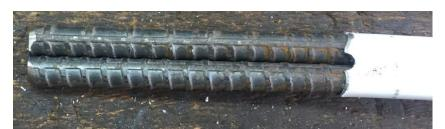
Then I used my grinding wheel to put bevels on the end.
